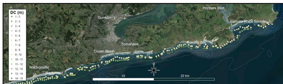
Figure 3.4: Brighton to Kaimata: DC minima and maxima for each transect location (coloured circles), and 5 m depth of material polygon in the modern sand wedge.
