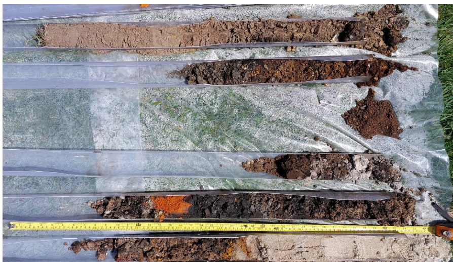
Photograph B9: Example of retrieved core, BH21. Ground level at top left, bottom of borehole at bottom right (taken 8.11.22).
