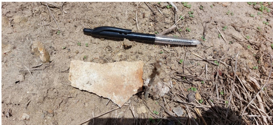
Photographs B7 (top) and B8 (bottom): Landfill materials such as brick, glass, concrete, timber, ash/charcoal and suspected ACM (shown in B8) daylighting on the bank south of the railway track, at the northern boundary of Kettle Park (taken 3.11.22).
