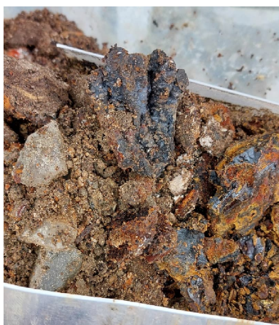
Photographs B15 (left) and B16 (right): Metallic forge/smelter waste at BH48 (left, taken 18.11.22) and BH38 (right taken 16.11.22).
