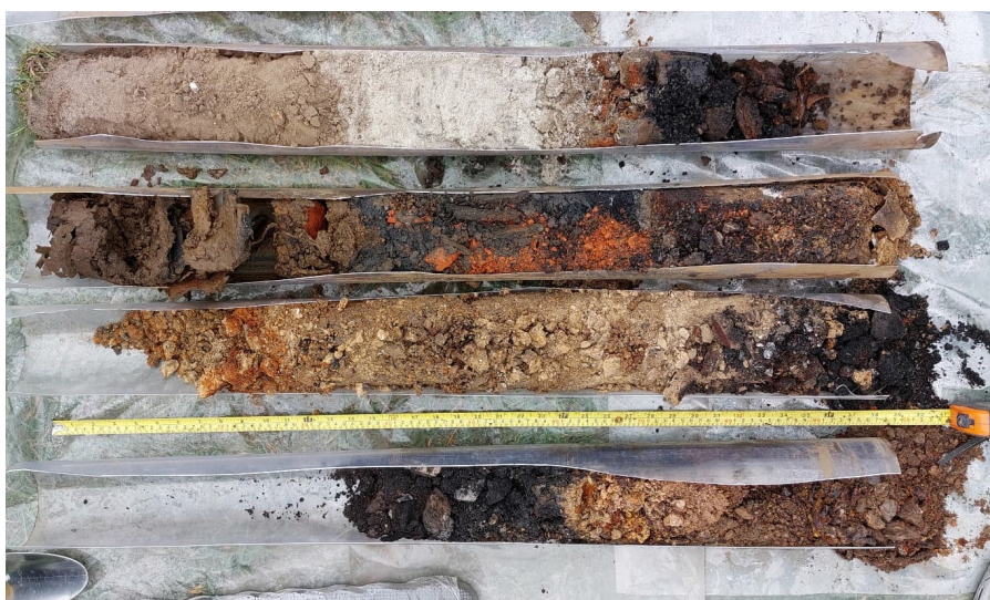
Photograph B10: Example of retrieved core, BH48. Ground level at top left, 4 m bgl at bottom right (taken 18.11.22).
