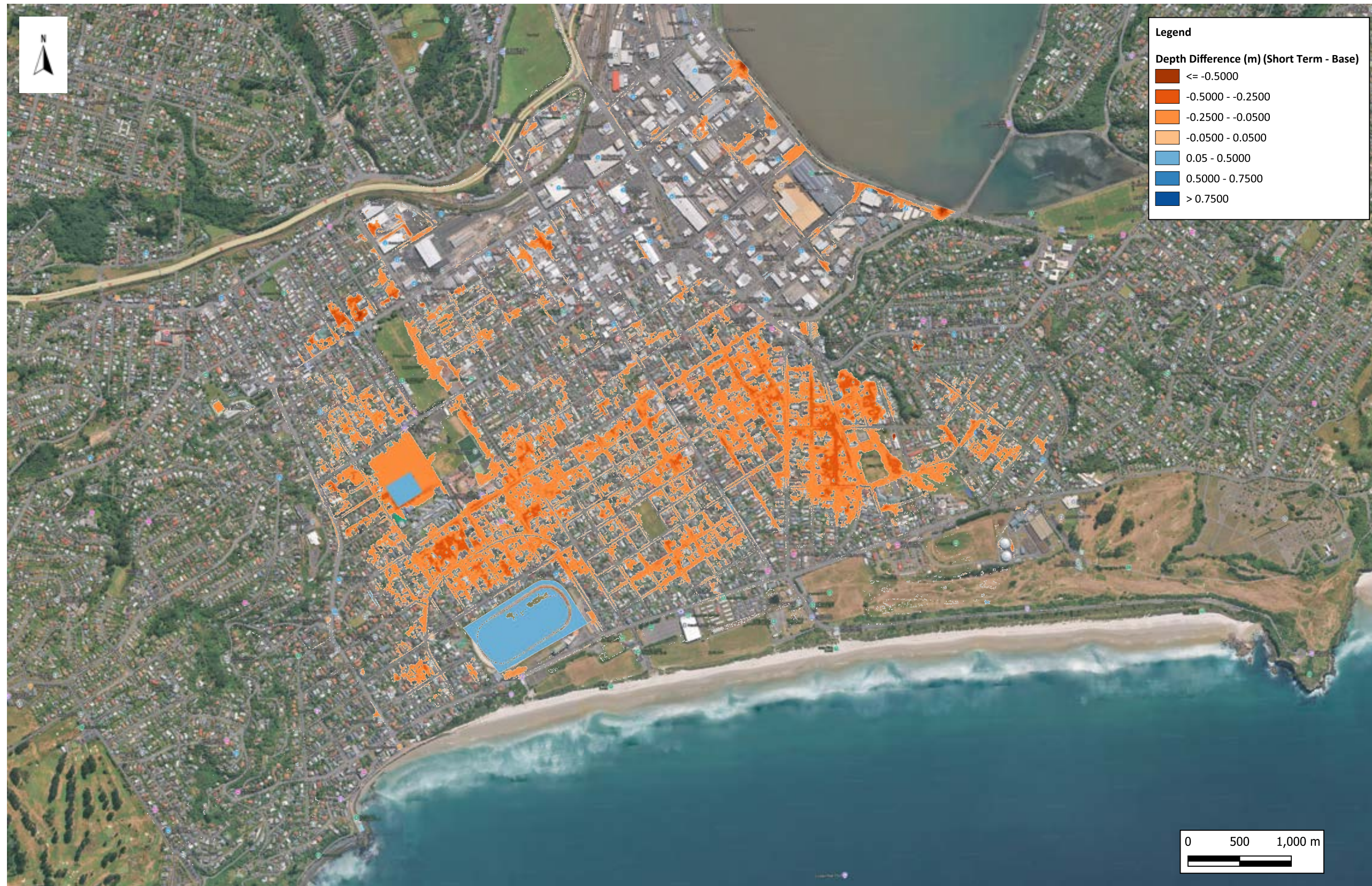
South Dunedin - Short Term Flood Depth Difference Map Between Short Term & Base (1 in 10 Year Design Storm)
