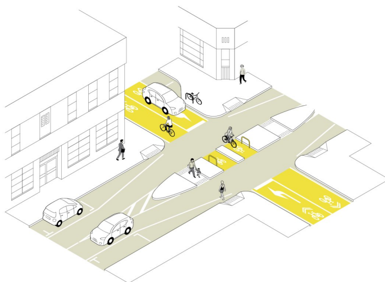
Figure 3: Cycle and pedestrian crossing at intersection restricts through traffic for motor vehicles while allowing people walking, wheeling and cycling to cross busy roads and continue along quieter streets.
